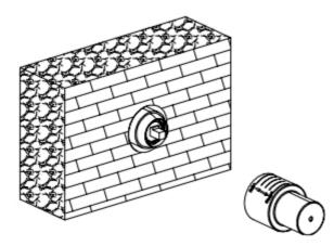
3. When the finished wall is complete, remove the protective cover.
