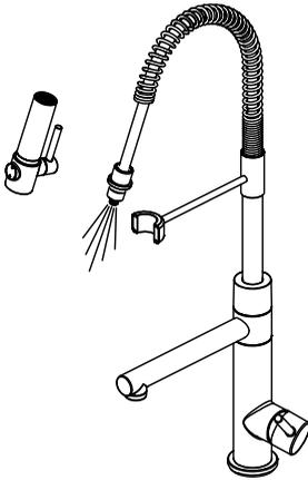
Pull the hose assembly out of the spout and remove the spray head by unscrewing it from the hose in a counterclockwise direction. Be sure to hold the end of the hose down into the sink and turn the faucet on to the warm position where it mixes hot and cold water.
