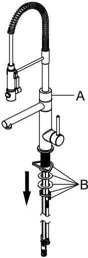
Shut off the water supply. Remove the old faucet. Clean the mounting surface. Remove mounting hardware (B) from faucet body (A).
