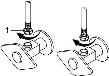
Thread the nut (1) on the supply line onto the outlet of the water supply valve and tighten with a wrench. Do not overtighten.
