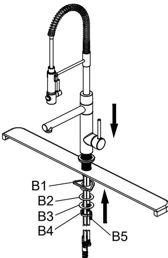
Insert faucet through hole in sink or countertop. From underneath sink, attach the seat (B1), rubber washer (B2), metal washer (B3), and nut (B4). Lock nut (B4) into position by tightening screws (B5).
