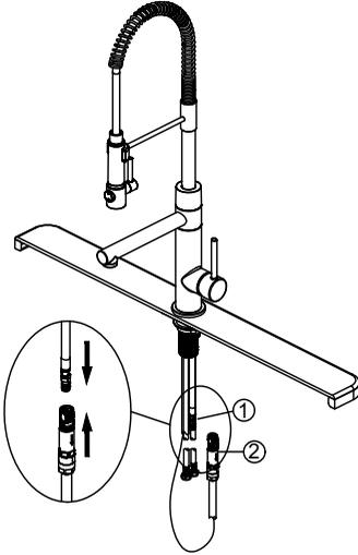
Push the quick connector (2) firmly upward and attach it to the receiving block (1). Pull down moderately to ensure the connection has been made.
