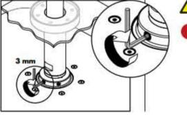
Tighten the safety screw using a 3 mm Allen wrench. Failure to tighten the safety screw may result in injury or product damage.
