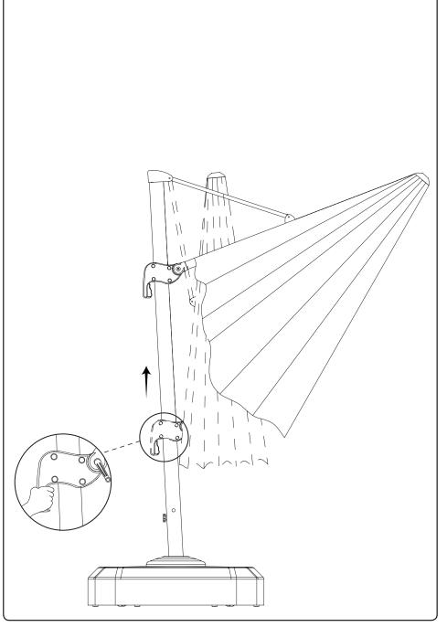
HAND CRANK OPERATION - (Note: be sure to remove all tape, foam or cardboard from the umbrella before opening.)
