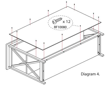
Step 4: Turn the back upright. Attach Back Panel into the unit by using 12 screws (RF10080) as per diagram 4.
