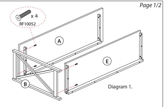
Step 1: Attach Table Top (A) and Bottom Shelf (E) to the Left Panel (B) by using 4 screws (RF10052) as per diagram 1.
