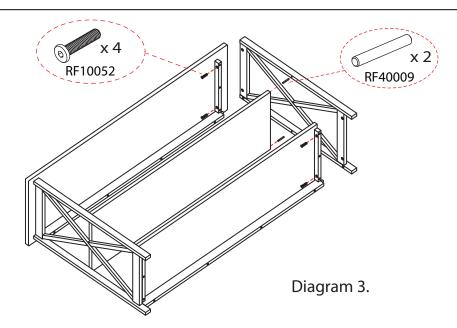
Step 3: Attach Right Panel (C) into the unit by using 2 Metal Pins (RF40009) and 4 screws (RF10052) as per diagram 3.
