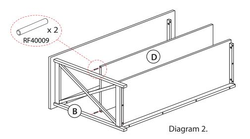
Step 2: Insert 2 Metal Pins (RF40009) into the edge of Middle Shelf (D), then put it into the unit at the holes on the Left Panel (B) as per diagram 2.
