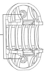
4 Fasten both 1" mounting bracket (B) and 7/8" mounting bracket (C) to the wall, using 2 mounting screws (E) each.
