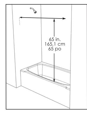
3 Drill the 2 marked spots for each mounting bracket. Insert drywall anchors (F) in the holes (unless screw will go directly into a stud).
