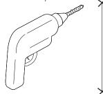
Note: use a 9/32 inch (7mm) drill bit for drywall anchor installation. Use a 5/64 inch (2mm) drill bit for direct stud installation.
