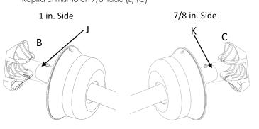
8 Screw in threaded pin screw(D) into pins on 1 inch side until tight
