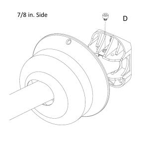
10 Tighten the 4 set screws on both brackets to level the rods.
