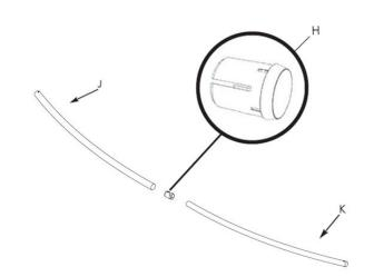
7 Align 1" rod(J) pins to center of bracket(B), compress pins and slide into1 in. mounting bracket (B) until pins open. Repeat same on 7/8" side (K) (C).
