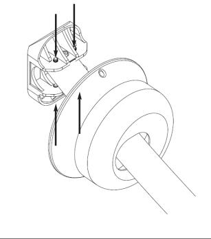
11 Attach decorative cover (A) using set screws (G) at the top and bottom using small allen wrench (I) as shown. Do this on both sides.
