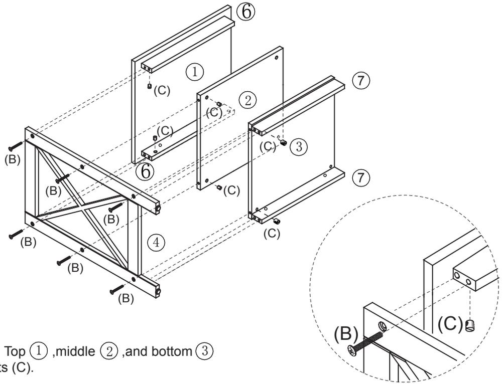
1. Carefully connect Left Panel (4) to Top (1), middle (2), and bottom (3) panels using Bolts (B) and Lock Nuts (C).
