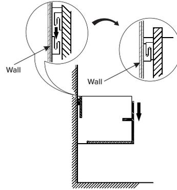
Align the preinstalled brackets on the back of the vanity to the previously installed wall brackets and hang the vanity.
