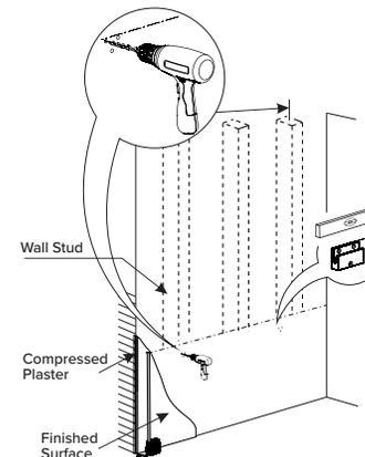
Use level to mark holes for mounting brackets, proceed to drill holes
