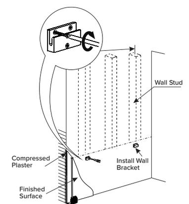
Install mounting brackets using screws provided. Proceed to Step 4.
