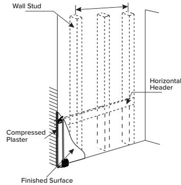
Install in-wall horizontal header at framing stage factoring in desired height of vanity, including vanity sink.
