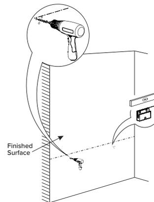
Use level to mark holes for mounting brackets, proceed to drill holes
