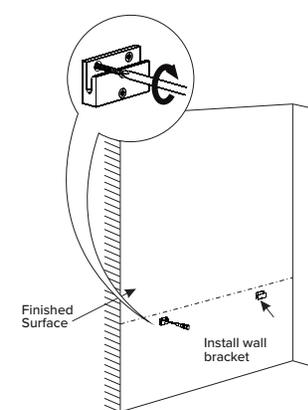
Install mounting brackets using screws provided. Proceed to Step 4.
