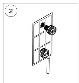
Insert the adjustable brass connectors and tighten until they are flush with the finished wall.
