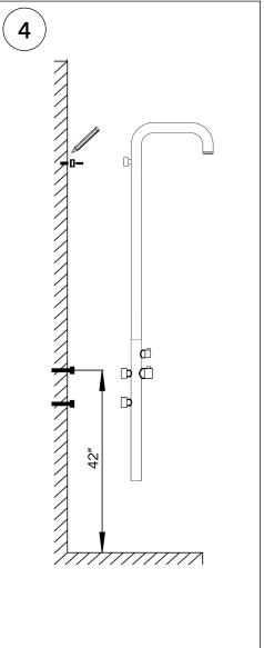
Hold the assembled fixture in place and mark the position of the upper bracket. Then, install the upper bracket.
