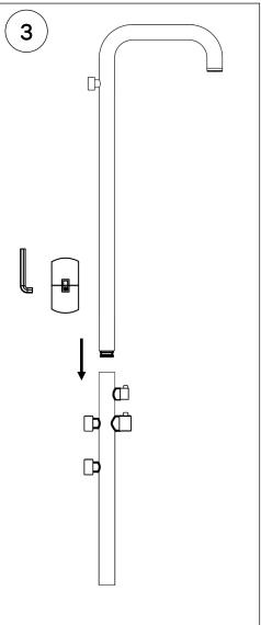
Assemble the fixture by inserting the upper part into the lower part. Align the indicator on the back of the fixture and tighten the set screw.
