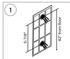
Install 1/2" hot & cold supplies at 42" height from the finished floor and 5-7/8" apart on center. Use the included NPT to G thread adapters and make sure the end of the adapter does not protrude from the finished wall.
